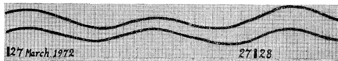
FIGURE 6. A sample of strainmeter records showing the effects of site inhomogeneity. The two instruments were approximately 500 m apart. Similar effects have been observed on instruments at separations of 2 m.
